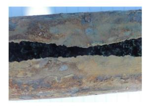
Photograph 2. Perforation of a rising main from corrosion
