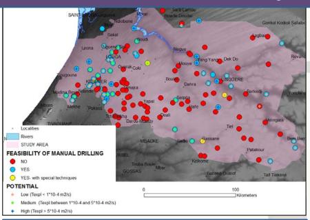
Estimating feasibility and potential for manual drilling at borehole positions
