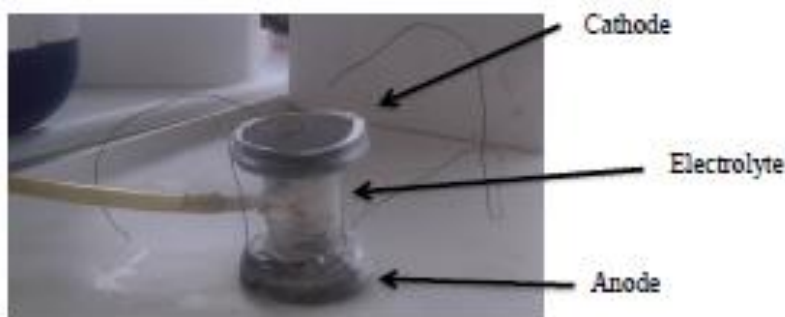
A photograph showing the glass reactor. Picture was taken in the laboratory before placing the reactor inside the aquarium.
