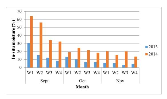
Figure 2b. In-situ moisture distribution in soils (before and after the construction of deep trenches at downstream of culverts in Megab area, Tigray, Ethiopia. Construction of the deep trench was done on June 2014. Monitoring was done for the period September-November for both years (2013 and 2014). (W1= Week one; W2=Week two; W3=Week three and W4=Week four).
