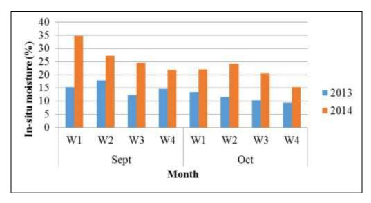
Figure 3b. In-situ moisture distribution in soils (before and after the construction of structures that divert runoff from culverts into farm lands along the Mekelle-Wukro road (Kihen), Tigray, Ethiopia. Construction of the diversion structures was done on May-June 2014. Monitoring was done for the period September-October for both years (2013 and 2014). (WI = Week one; W2=Week two; W3=Week three and W4=Week four).
