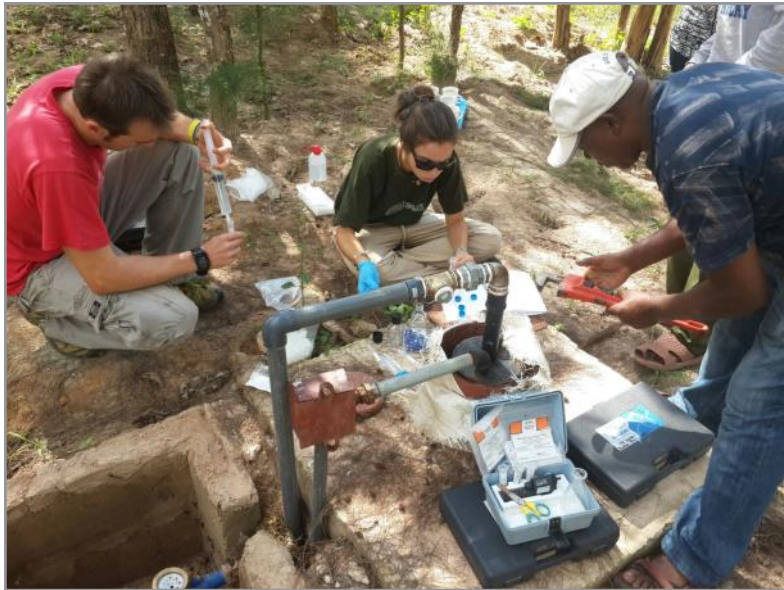
Research Team collects samples from a borehole during the first groundwater sampling campaign in Sep – Oct 2015
