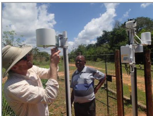
TAHMO Engineer (Zack) & KMS Director Kwale (Dominic) Installing AWS at Kidonge Gate, Shimba Hills National Reserve
