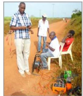
WRMA's Geophysics field team with 2D tomography equipment
