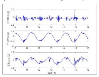
cost accelerometer embedded in the pump handle. **3-axis acceleration of Afridev pump handle.**
