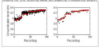
Measured depth [red] vs. predicted depth [black] by spline [left] and by recording [right].
