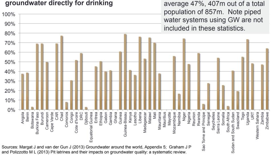
47% of the population of the region use groundwater directly from springs, wells and boreholes, the vast majority of these using handpumps.
