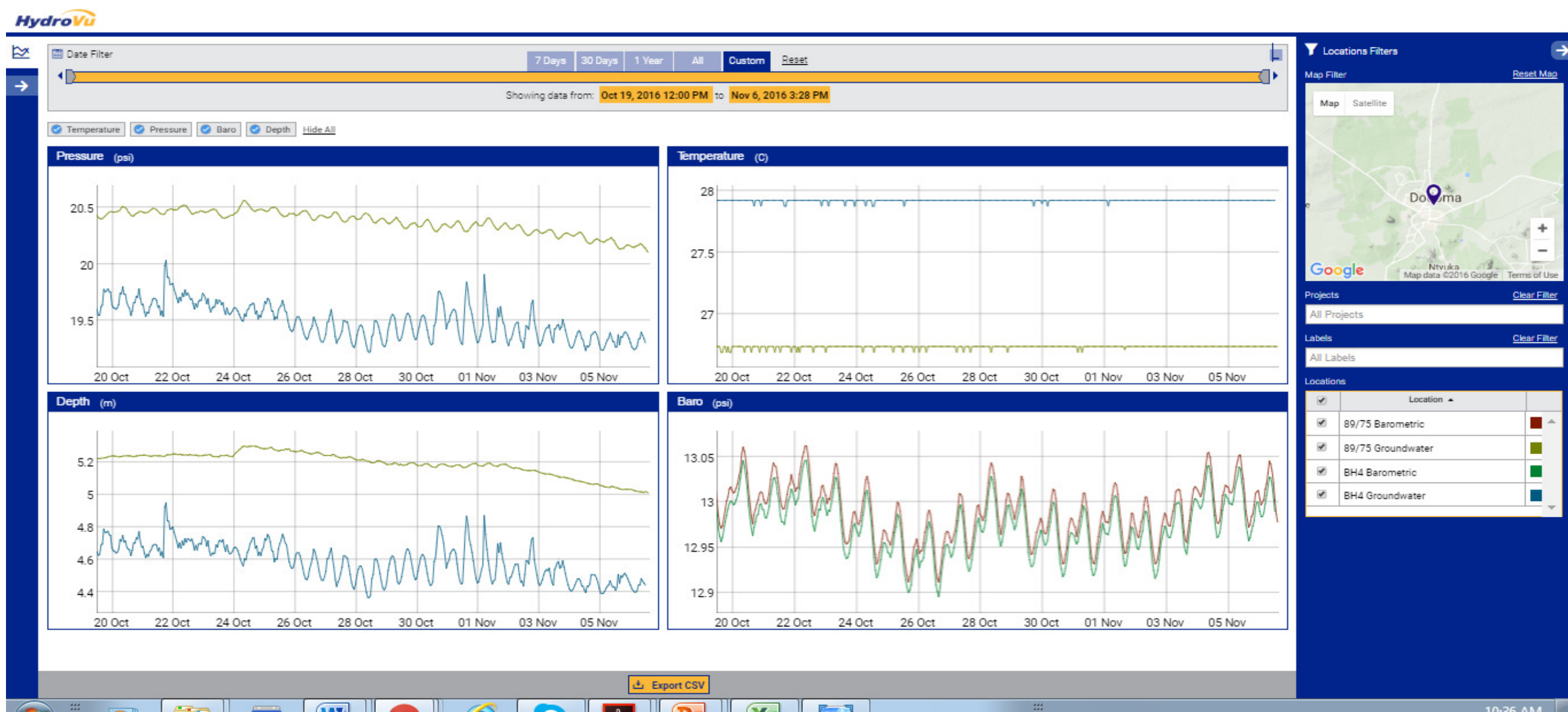
Figure 3. High-frequency (hourly) monitoring of groundwater using in situ data loggers and telemetry.
