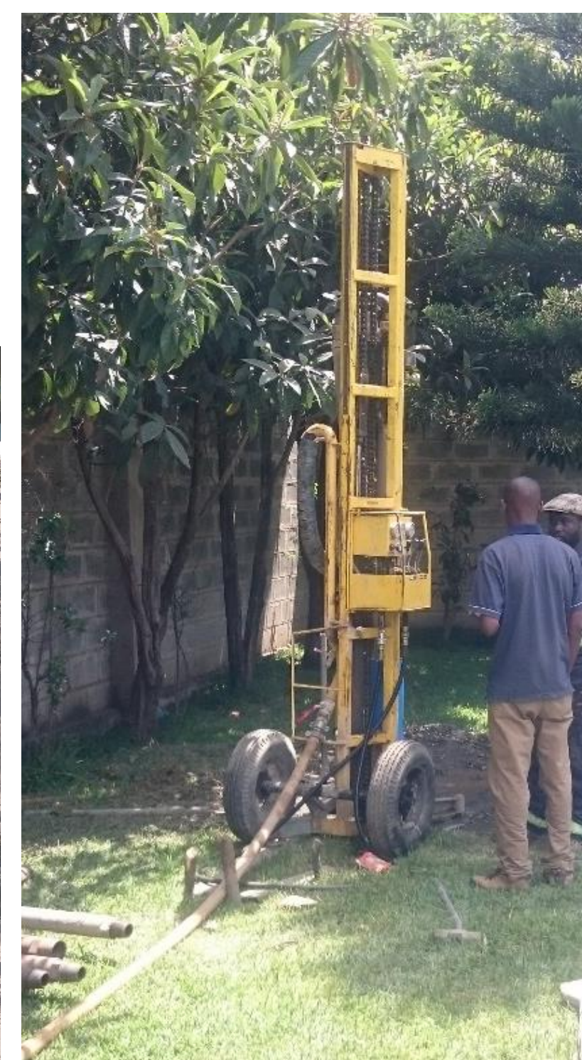
Example of ERT section (upper left); PAT-301 drilling rig used (right); At this location, we drilled 3 separate wells of various depths (5, 15, and 25m; lower left)
