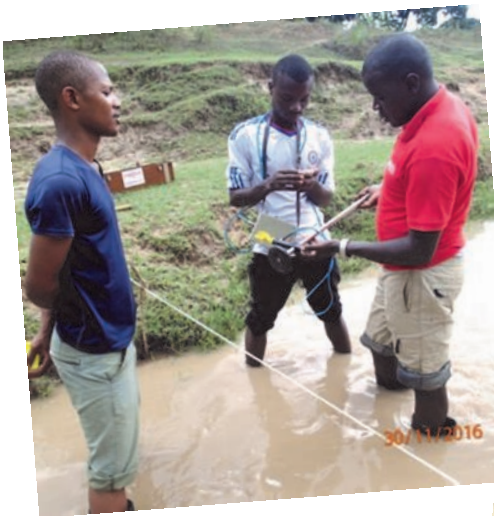
Flow Measurement on Ramisi River at Eshu Bridge during short rains in November 2017 using Current Velocity Meter
