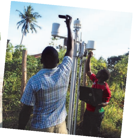
Gilbert of TAHMO undertaking regular maintenance of the AWS at Kidongo Gate in Shimba Hills
