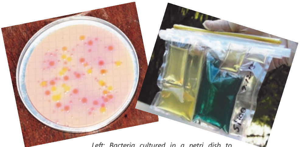
Left: Bacteria cultured in a petri dish to investigate groundwater contamination; Right: Test kit bag showing colour change on presence of E. Coli (Photo: Aquagenx)
