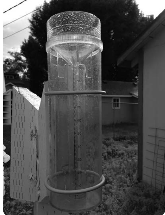
Standard rain gauge. 4-inch plastic rain gauge, typical of those used by the CoCoRaHS program, photo by Famartin, CC BY 3.0 . Wikimedia Commons.
