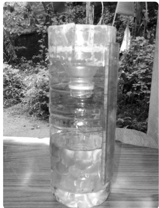
Rain gauge made by students. Photo by Fotokannan, CC BY 3.0 . Wikimedia Commons.
